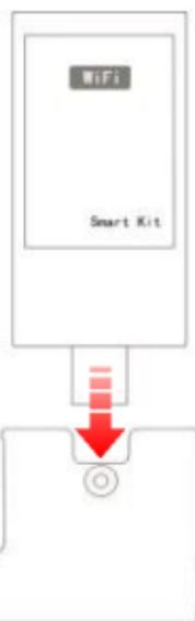
Open the panel to find installation port on the right side, Loosen this screw and take out the plug, then insert the Smart Kit as shown in picture. (Note: please put the side with "Smart Kit" in front)
