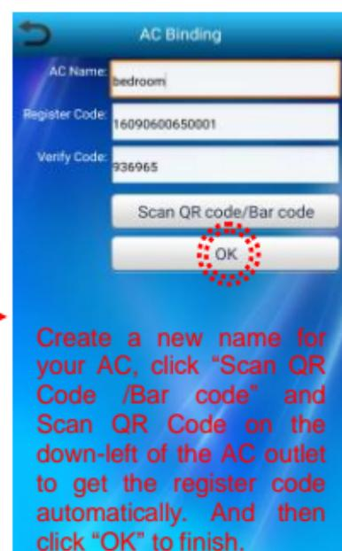
Create a new name for your AC, click "Scan QR Code /Bar code" and Scan QR Code on the down-left of the AC outlet to get the register code automatically. And then click "OK" to finish.
