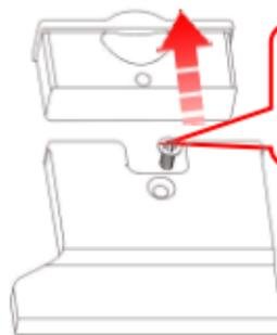
Loosen this screw, take out the plug and insert the "Smart Kit" .
