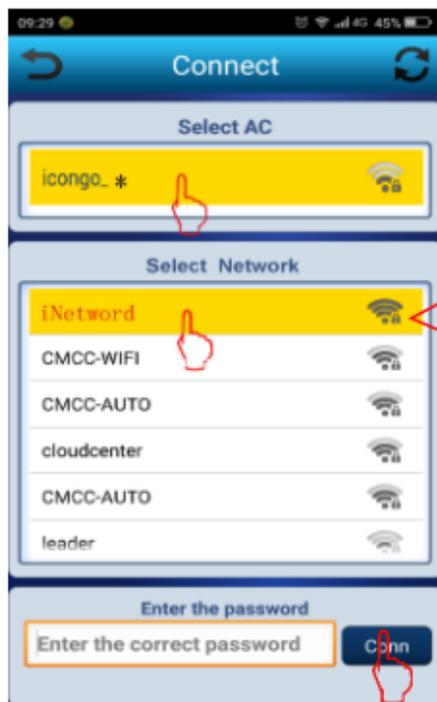
Select an air conditioner to be connected to network (default AC name is icongo\_\*). Select a network and input password. Click "Conn" to finish setting.
